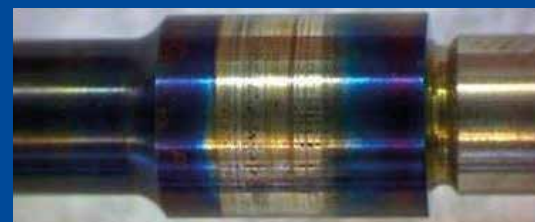
Evidence of overheating, caused by oil starvation
