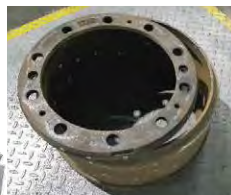
Failed aftermarket Scania drum ref; DVSA investigation Jan 20
